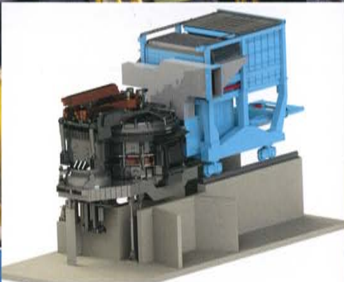
Scrap preheating and charging system
